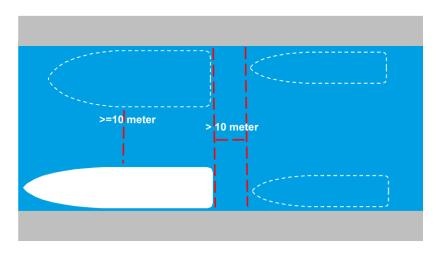
Measurement of distances before or behind (left) and on all sides (right)
